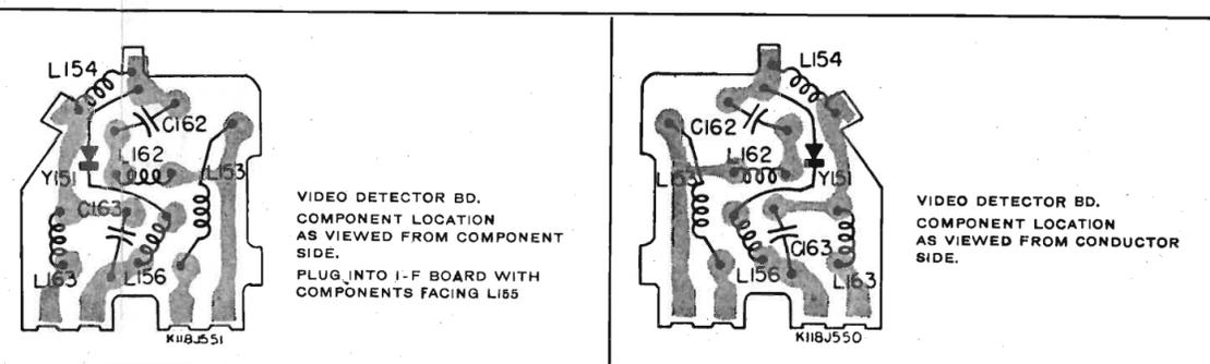
VIDEO DETECTOR BD. COMPONENT LOCATION AS VIEWED FROM COMPONENT SIDE. PLUG INTO I-F BOARD WITH COMPONENTS FACING L155
